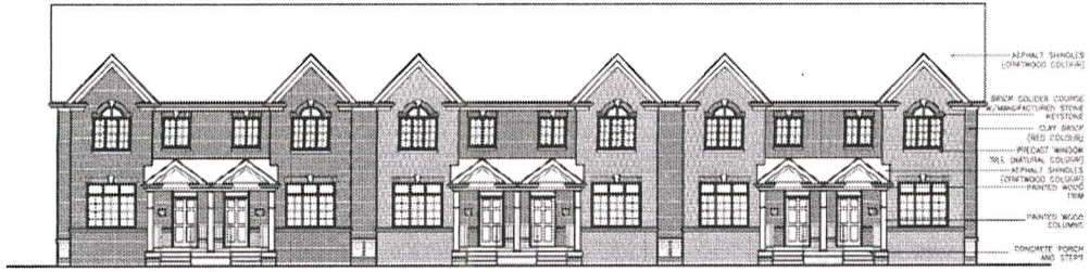
TYPICAL TOWNHOUSE ELEVATION FROM EAGLE ST. SCALE 1:100
